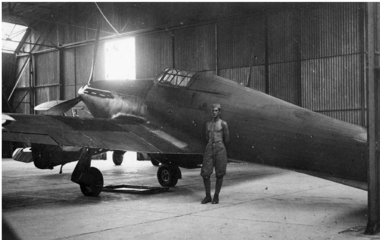
Hot day in one of the Borongaj hangars during the summer of 1940. Mechanic Relja Nedić posing in front of the Hurricane from the 2nd imported batch from Britain. Metal covered wings and armored windshield are clearly visible. There is a great possibility that the machine in the photo is 2314 that was involved in a tragic flying accident with a Bf 108 Taifun on 19 June 1940. Note the freshly painted part of the port wing, leading edge and wing root. (Dragan Kolundžić)
