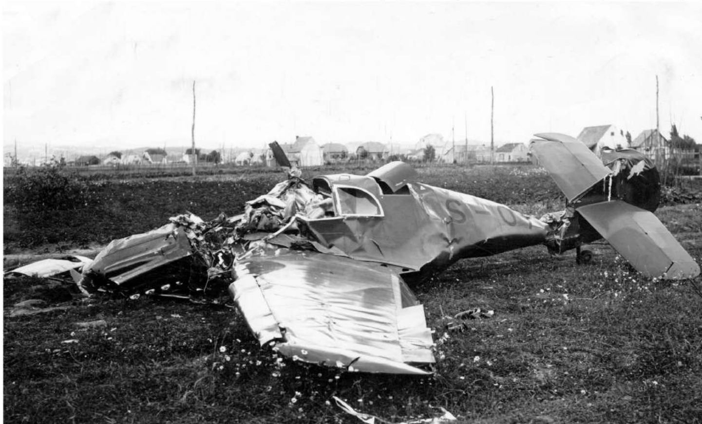
Sad remains of the VVKJ Bf 108 Taifun 5-07 (Nº777) at the Borongaj airport in Zagreb on 19 June 1940. Hurricane 2314 basically crushed the small aircraft when both were in their landing pattern at the same time. Lack of radio equipment and any other visible means of warning created the accident when the 108 flew right inside the Hurricane's blind spot. Taifun occupants, fighter pilot nar Čavić and pilot nar Marindolac were killed instantly. (Vladimir Bosner Jr.)
