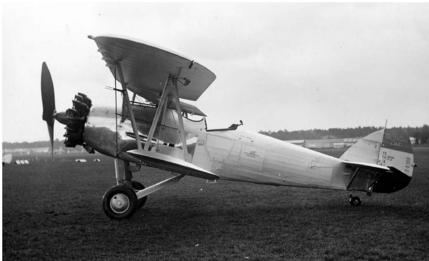
Yugoslav Hind №3 photographed at Brooklands during performance tests. №3 was intended as an experimental/development platform from the beginning. It was powered by a French Gnome et Rhône 9K Mistral (700hp) engine. It was delivered with an uncovered engine and open cabin with windshields, but, at the request of the VVKJ, it was heavily modified at the Zmaj airplane factory. This unique airplane was destroyed during the April war. (Djordje Nikolić)
