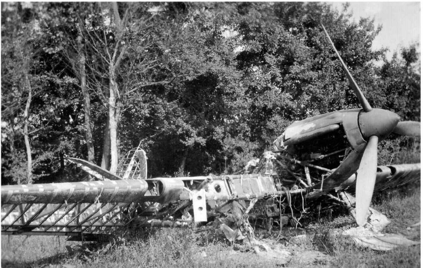
Completely burned out Hurricane Mk.I from 4.FR at the auxiliary airfield Bosanski Aleksandrovac. The wing clearly shows British build machine from the first imported batch. The propeller was changed at some point with a three bladed one. There is a huge possibility that Rogožarski U-21 propeller was used, because of nonstandard size of spinner that looks very similar to later Mk.II's. Photo was taken by a 1.Bomber Regiment observer during retreat. (Author)
