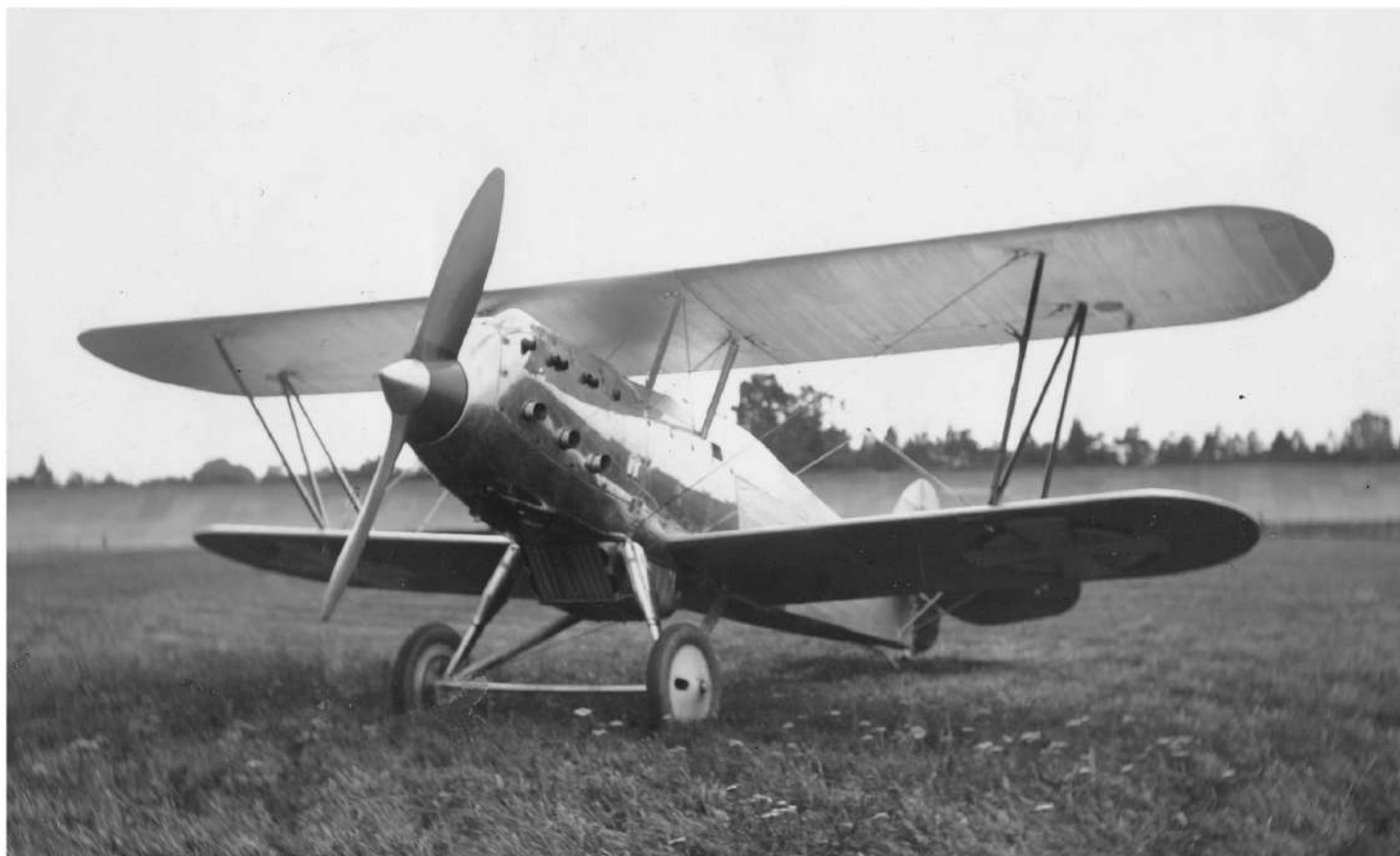
The third Hawker Fury Mk I for Royal Yugoslav Army Air Force equipped with a French built Hispano-Suiza (HS 12Nb) engine arrived in the Kingdom of Yugoslavia during November 1931. Although the Hispano engine had more power in comparison with the original Rolls Royce, the lack of a compressor in the French engine resulted in a disappointing performance. Here seen at Brooklands just before delivery (October/November 1931). (Djordje Nikolić)
