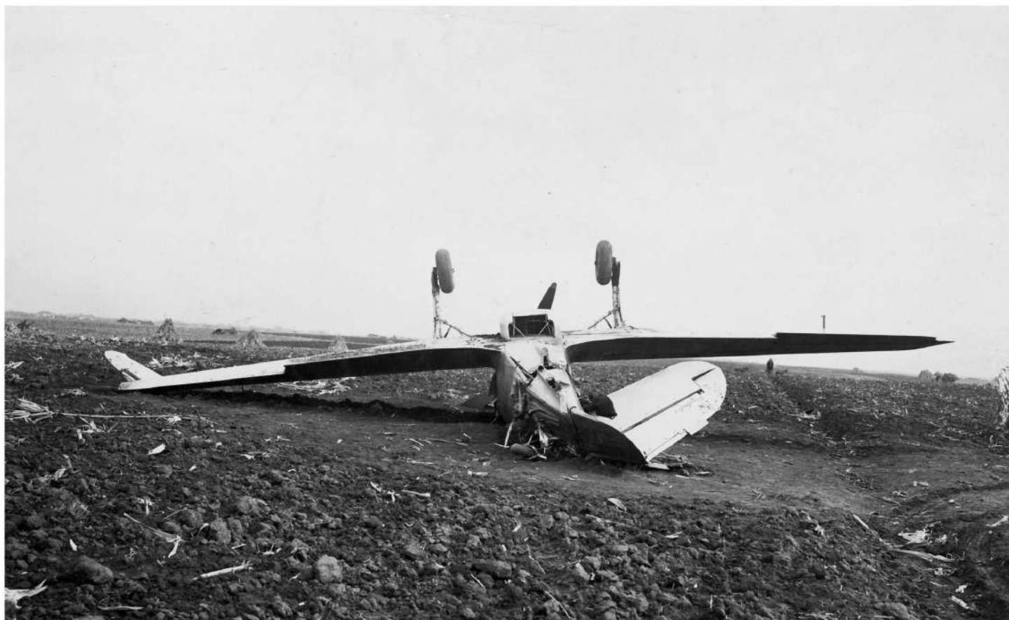
Hurricane Mk.I 2307 overturned in a field at Velika Krsna village. The extended landing gear was the reason why nar Vićovac lost his life in the accident. He actually broke his neck. The airplane was dismantled that same day by technicians from Belgrade, loaded onto Air Force Praga trucks and then reloaded onto a train in the nearby Mladenovac. It was repaired in a couple of months at Zmaj airplane factory and returned to active service. (Aleksandar Smiljanić)
