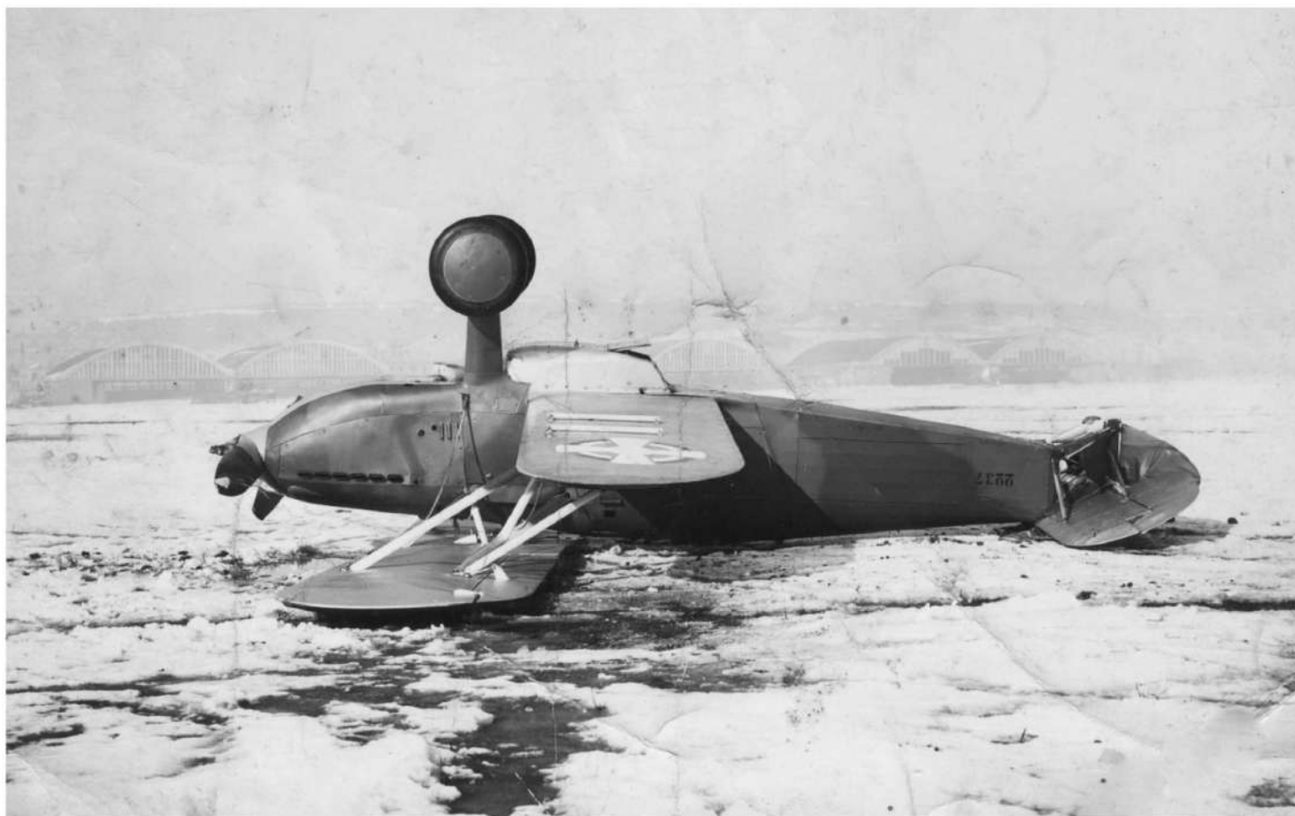
Nar Vasilije I. Vračević's landing accident with Fury Mk.II 2237 at the snow covered airstrip of Zagreb aerodrome, during the winter of 1939. Soft snow caused the aircraft to overturn. Absence of white code number on the fuselage is strange and deviates from VVKJ practice. Pilot Vračević remained unharmed, but would be less lucky on 27 Nov 1947, as a crew member of a military Lisunov Li-2, which crashed at Rumija Mountain killing all aboard. (Dragan Petrović)
